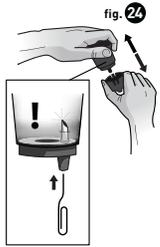
using the two front ribs as a guide, and snap them into place from the top.
